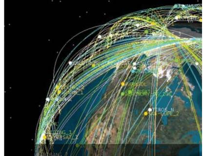
Thanks to the laws of orbital mechanics and the fact that most LEO satellites and other objects use midto high-inclination orbits, population density is lowest at the equator and highest near the poles.
