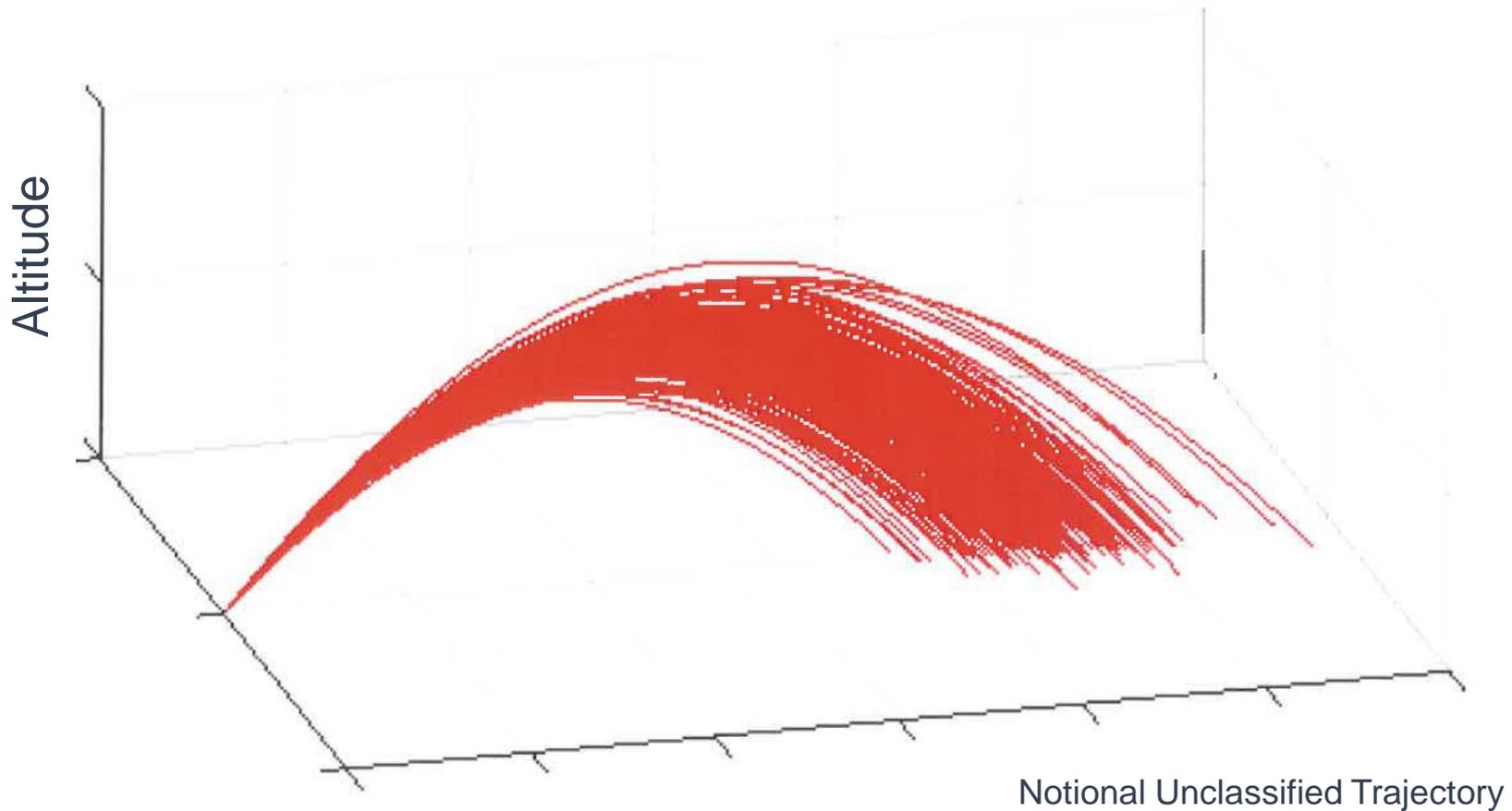
Monte Carlo set of trajectories that account for expected dispersions due to variations in parameters such as vehicle performance and atmospheric conditions
