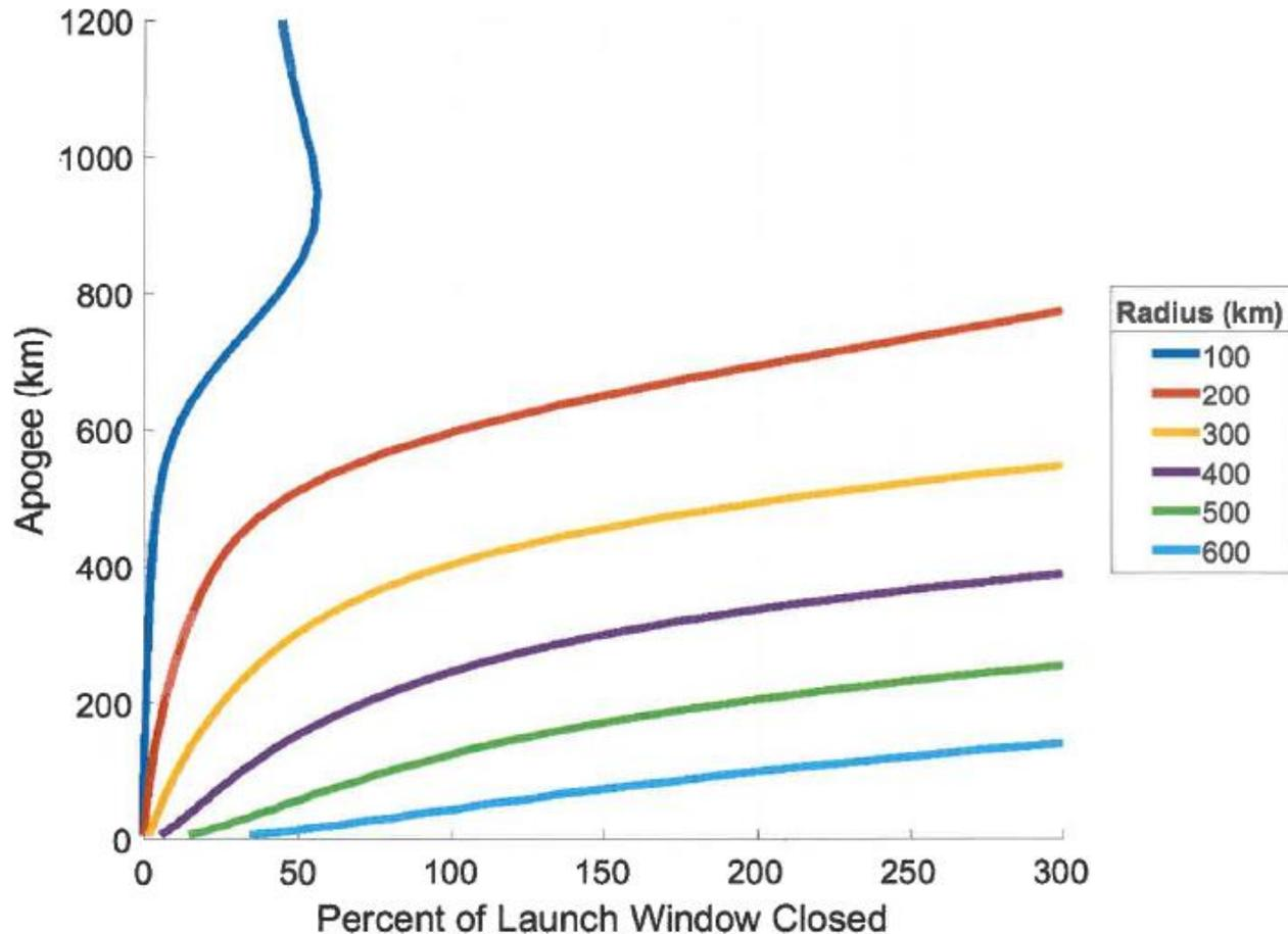
LW closure for a single screening volume. Following a ballistic trajectory with 45° launch elevation, with initial speed varied
