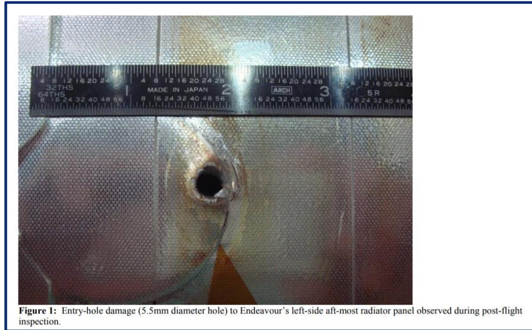
**Figure 1:** Entry-hole damage (5.5mm diameter hole) to Endeavour's left-side aft-most radiator panel observed during post-flight inspection.
