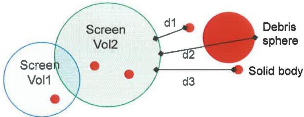
Adding  $d2$  to both screening volumes in this example is a simple (but over-conservative) way to ensure that the constraint is met
