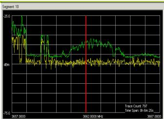
CF: 3662.0000MHz Span: 10.0000MHz ResBW: 12.210 kHz dB/div: 5 Ref. Level: -25.00dBm Vid Avg: 10 Beacon Correction: disabled
